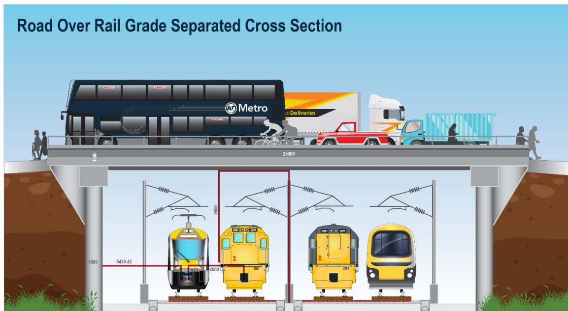
Figure 14-1: Road over Rail typical cross section
