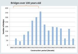
Figure 4: Age profile of rail network bridges
