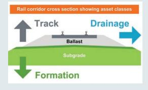
Figure 3: Cross section of assets in rail corridor
