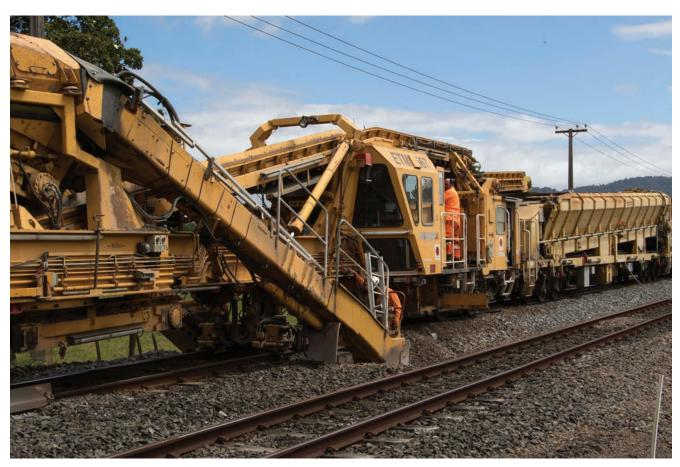
Ballast cleaners (above) and stabilisers (below) are important tools used to maintain the network.
